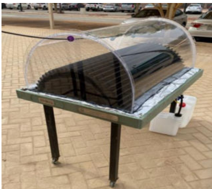
Fig. 3. V-Corrugated absorber solar still prototype.
