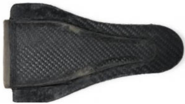
Fig. 2. final part after attempting to demold it from the printed mold
