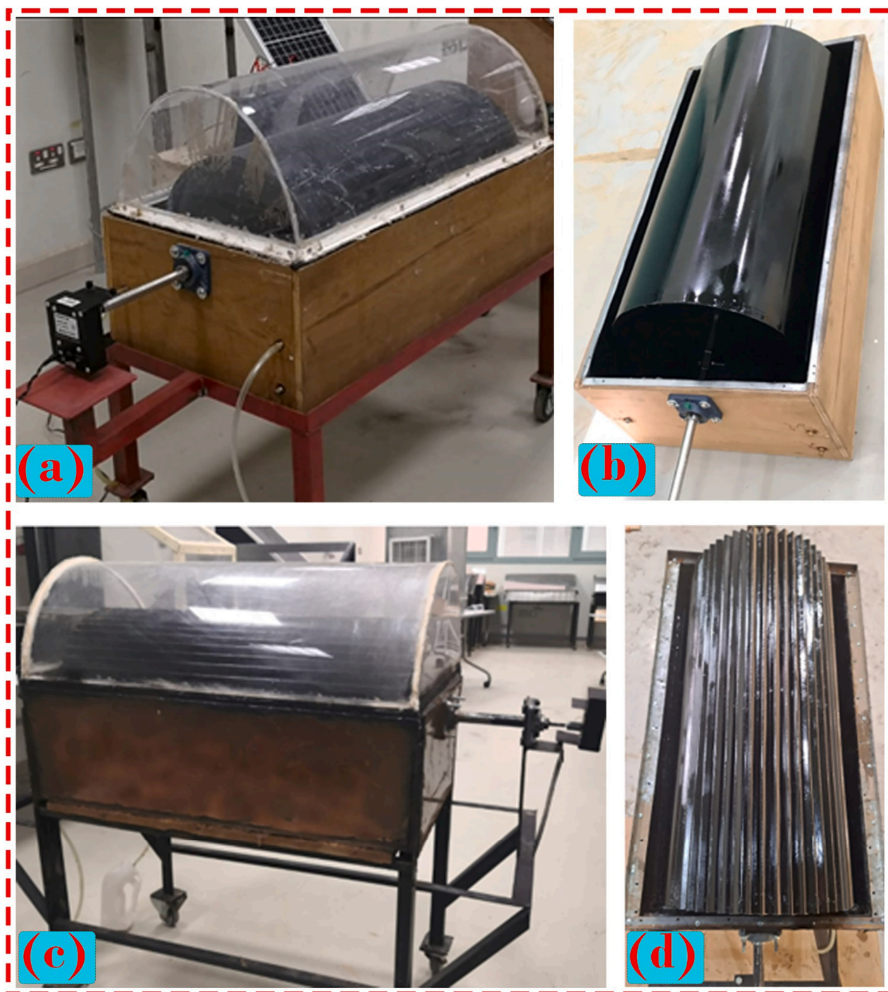
Fig. 1. Photographs of the investigated solar stills: (a) conventional drum solar still (DSS), (b) conventional drum, (c) corrugated drum solar still (CDSS), and (d) corrugated drum.
