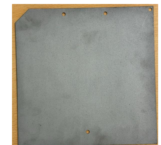
Titanium Coated with 1μm platinum
