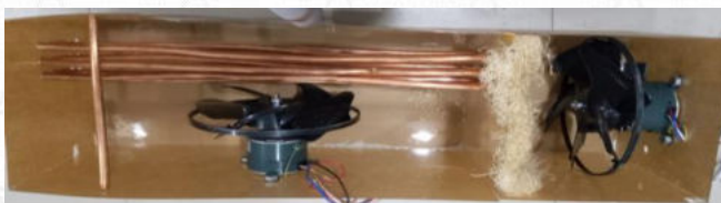
Figure 5. The top view of the IEC case shows the fan, heat exchanger, and wetted pad.
