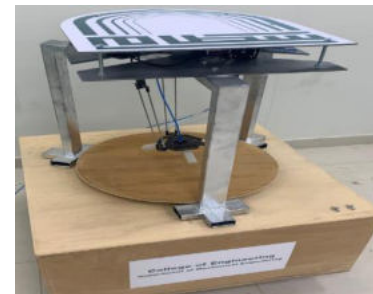
Fig. 7. Project prototype when assembly delta robot manipulator with end-effector
